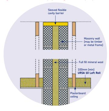
Figure 11 - Roof Junction (separating wall/room in roof)
