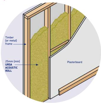
Figure 4 - Timber Frame Separating Wall
