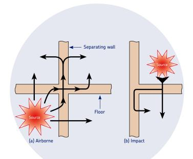
Figure 2 - Flanking Sound Transmission
